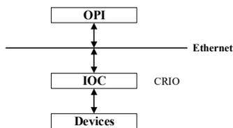
Figure 1: The structure of vacuum control system.
