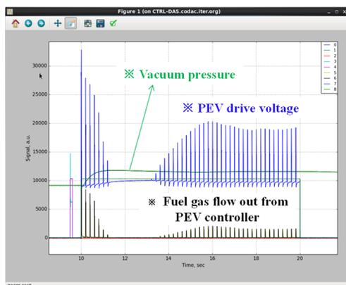
Figure 6: Feasibility check through the vacuum pressure control. Chop the control signal to cope with the slow response time on the pressure sensor.
