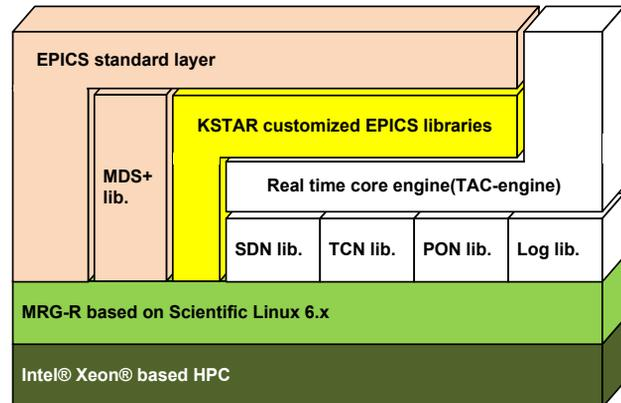
Figure 1: Software Components and architecture of EPICS IOC for real time processing.
