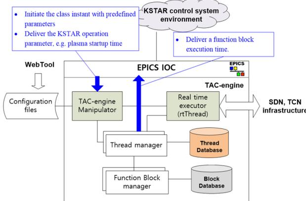
Figure 3: Basic software components and connections inside EPICS IOC.
