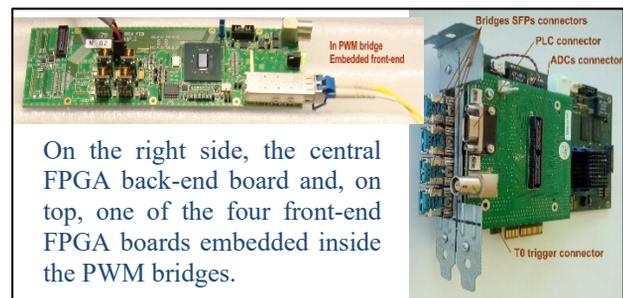
Figure 2: Real time control hardware.
