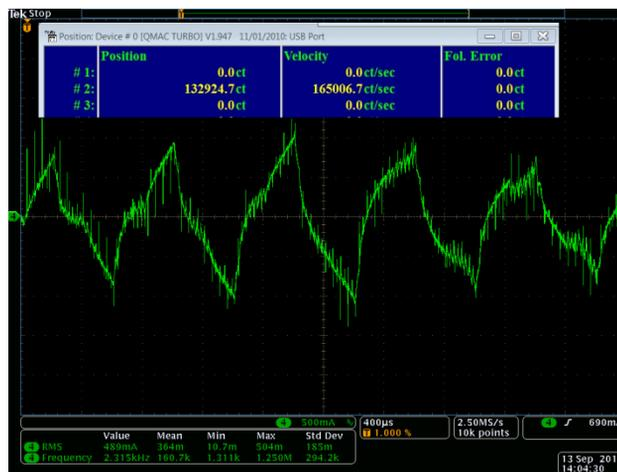
Figure 7: MFA-PP current trace, Ixx22=165 (rated speed), Ixx77=200, Ixx61=0.003; PeWin executed motion at 165 ct/ms.
