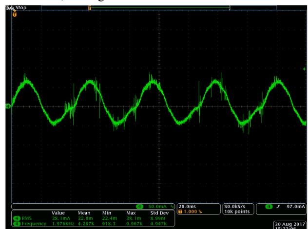
Figure 4: 125 mA stepper current trace, Ixx22=5, Ixx77=100, Ixx61=0.01.
