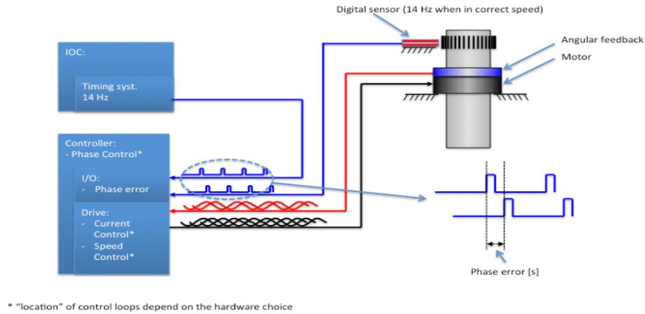
Figure 2: Equipment foreseen to control the target wheel.
