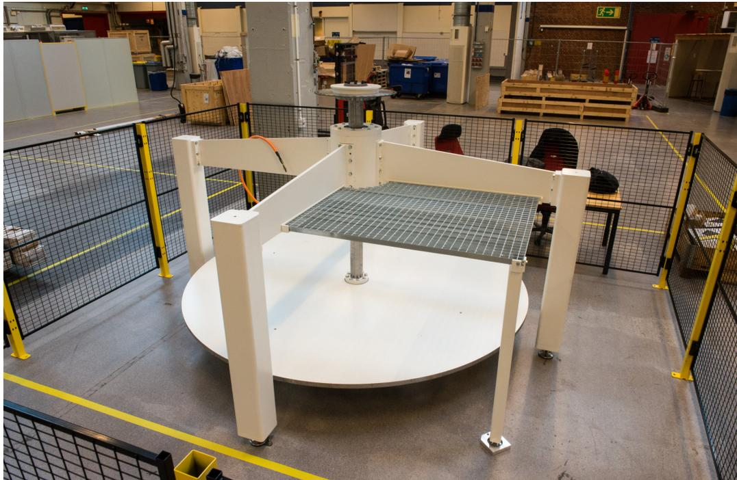
Figure 4: The target wheel motion control test assembly.
