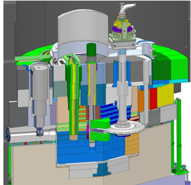
Figure 1: CAD model of the ESS Target, showing the target wheel, moderator and other components within the monolith.
