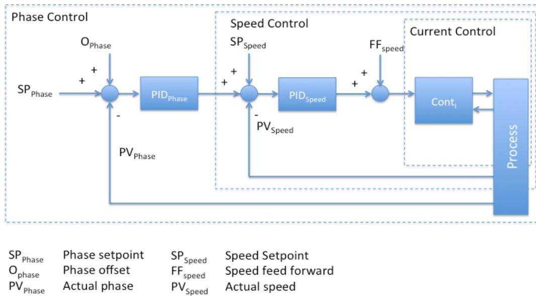
Figure 3: Cascaded control loops.
