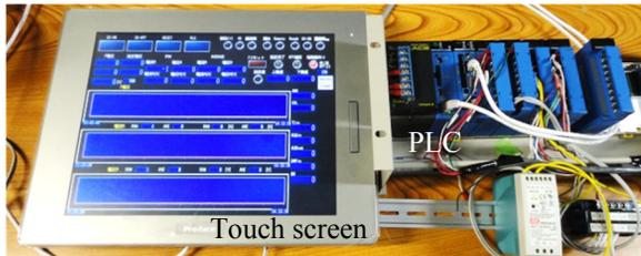
Figure 3: Photograph of PLC and touch screen.
