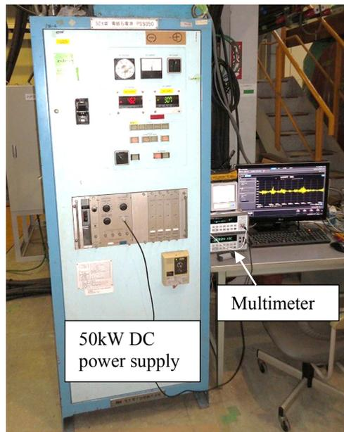
Figure 4: Photograph of thyristor power supply and multimeter.
