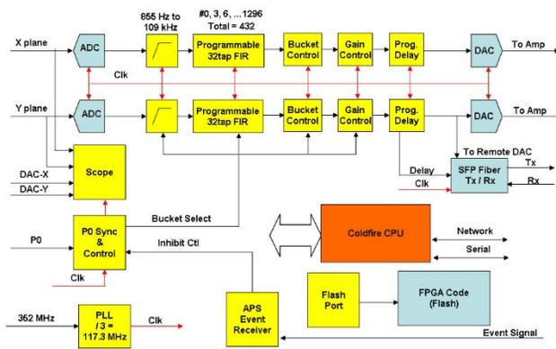
Figure 2: FPGA block diagram of the P0 feedback.
