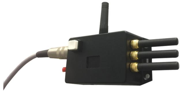
Figure 4: First generation operational node. External connector cable seen at left for RS-232 interface and external power. Internal 3xAAA battery holder for wireless operation is provided.
