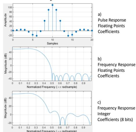
Figure 3: Graphs from the System Generator GUI during the design of the digital low pass FIR Filters.
