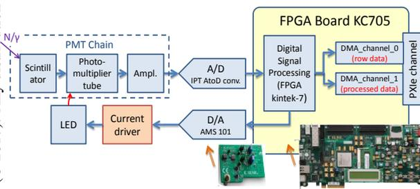
Figure 1: Scheme of the hardware proposed for the PMT chain gain calibration system.
