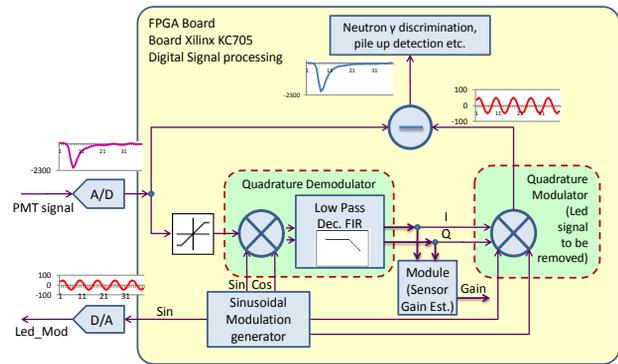
Figure 2: Fully Digital implementation for the calibration for the PMT chain gain, based on Intensity LED Modulation.
