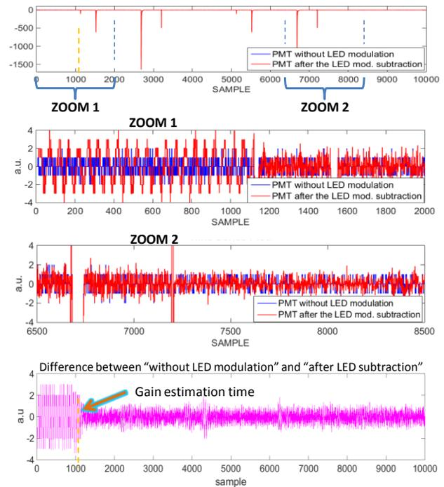
Figure 7: Analysis of the PMT signal: without the addition of LED modulation (blue) and after the LED modulation signal cancellation (red). Difference between the two signals, which corresponds to the noise introduced by the calibration system (pink).
