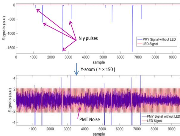
Figure 4: Simulation signals for PMT and LED modulation.
