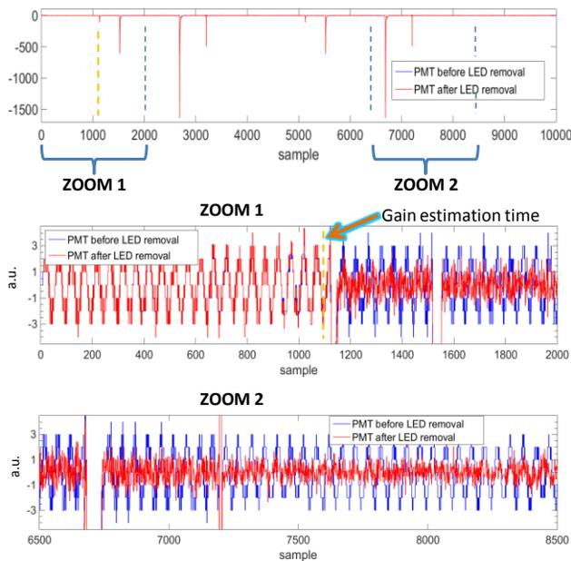
Figure 6: Pulse before and after LED removal.
