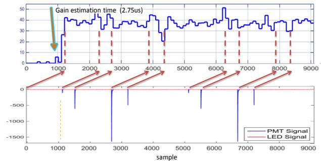
Figure 5: PMT Chain Gain estimation.
