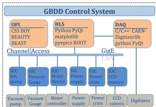
Figure 2: The software architecture for GBDD CS.
