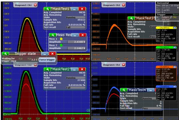
Figure 5: Kicker pulse monitoring system. In this event, one kicker fired a second time while re-charging.
