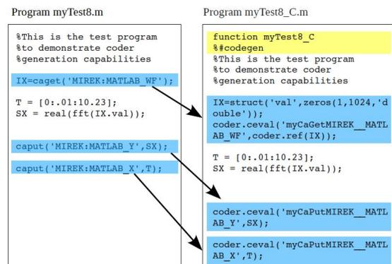
Figure 3: The original myTest8.m program and its pre-processing result.
