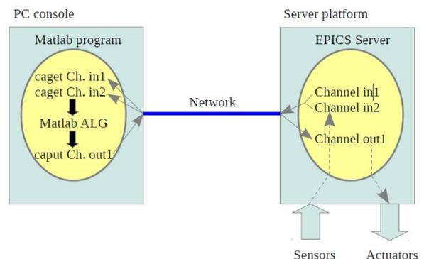
Figure 1: Closed loop controls with the use of an EPICS CA server and a MATLAB program.
