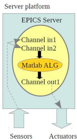
Figure 2: MATLAB algorithms embedded into the IOC.
