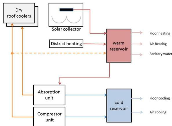
Figure 5: B774 energy flow principle.
