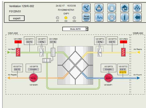
Figure 2: Example of control panel interface component.
