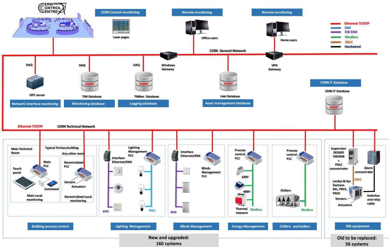
Figure 3: Control & monitoring architecture of the CERN tertiary building infrastructure.
