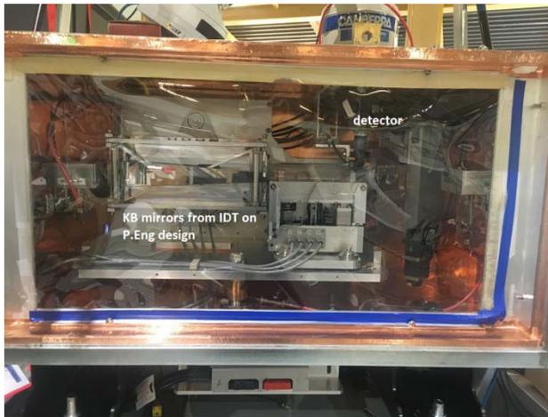
Figure: 3 TES End Station sample chamber, contains (from left to right, along beam path) I-zero ion chamber, custom KB mirror system, sample stage, visible-light camera, detectors, and transmission ion chamber.
