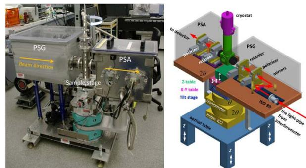
Figure 7: Müller-Matrix ellipsometer with Polarization State Generator (PSG) and Polarization State Analyser (PSA) [6].
