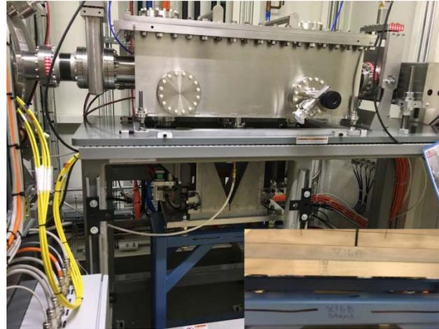
Figure 4: Vertical collimating mirror reassembled from two identical mirror systems recovered from X16A and X16B.
