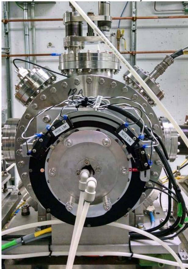
Figure 6: QAS Monochromator retrofitted with Direct Drive servomotor from NIKKI DENSO.
