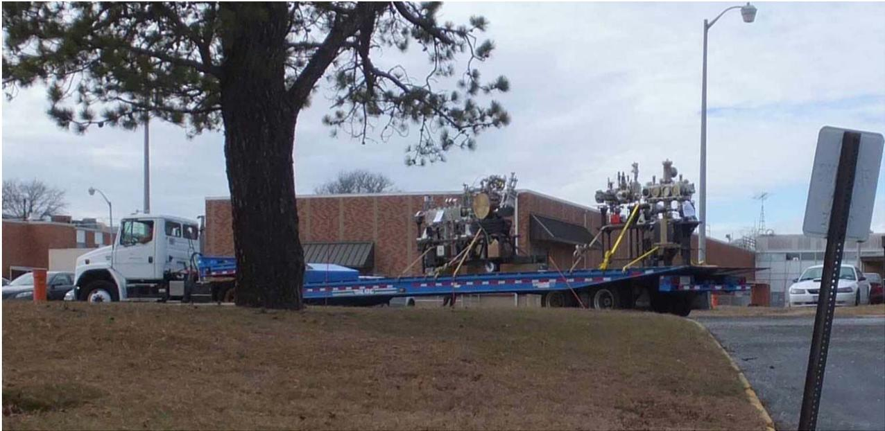
Figure 1: Components of NSLS X15B being moved to NSLS-II 8-BM. From left to right: focusing mirror, monochromator, vertically collimating mirror, beam-defining slits.
