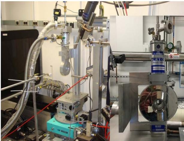
Figure 8: 5K cryostat on the left, and superconducting 5T magnet on the right, both from Cryo Industries of America (CIA), to be combined in a unique sample environment.
