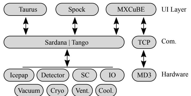
Figure 4: Simplified structure of the control system describing how the different elements are related.
