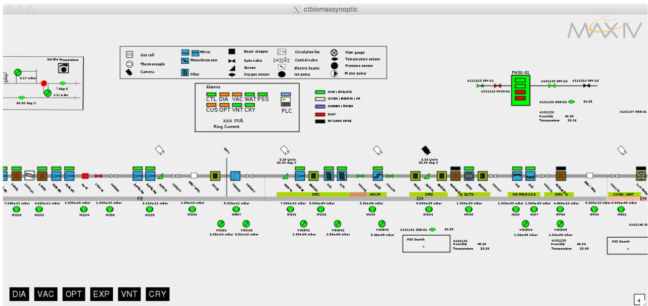
Figure 3: BioMAX beamline synoptic, a graphical interface describing the status of the main devices of the beamline. Users can hover and click on elements and the corresponding device panel is displayed.
