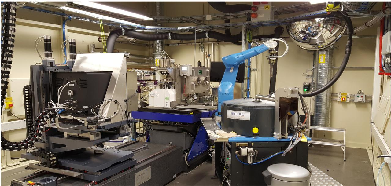
Figure 1: BioMAX experimental station; from left to right: EIGER 16M detector and its support table, MD3 diffractometer and the Beam Conditioning Unit (BCU) on their table, ISARA Sample Changer.
