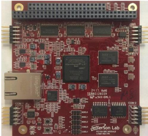
Figure 2: The Picture of the SoC IOC Board.
