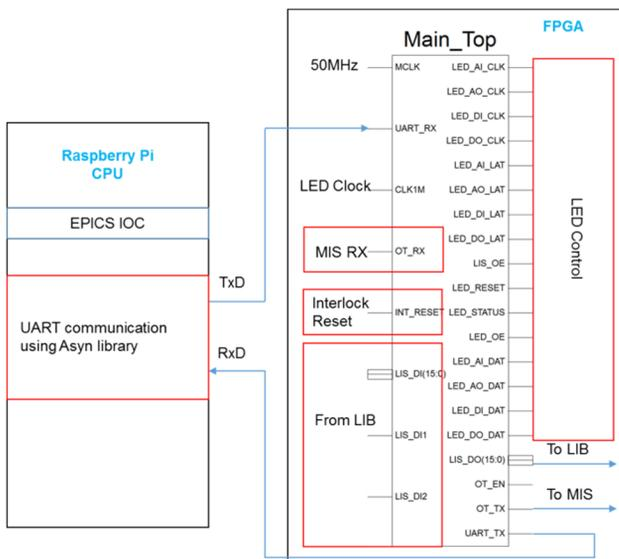
Figure 2: Architecture of MPS hardware.
