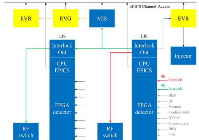
Figure 3: Schematic diagram for loopback test of LIS (a) Red line) and MIS (b) Green line).
