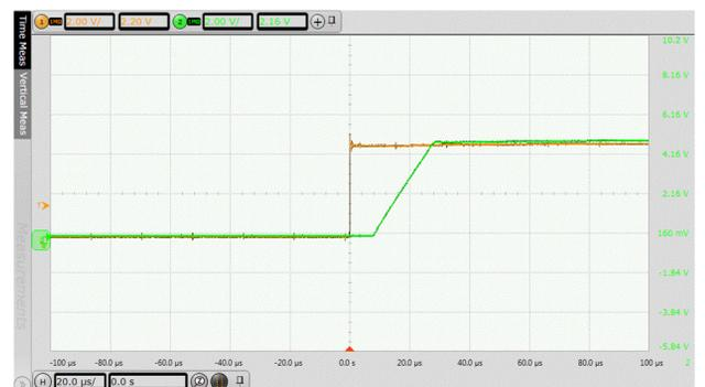
Figure 4: Response time of LIS loopback (Orange: Interlock Input, Green: Interlock Output).
