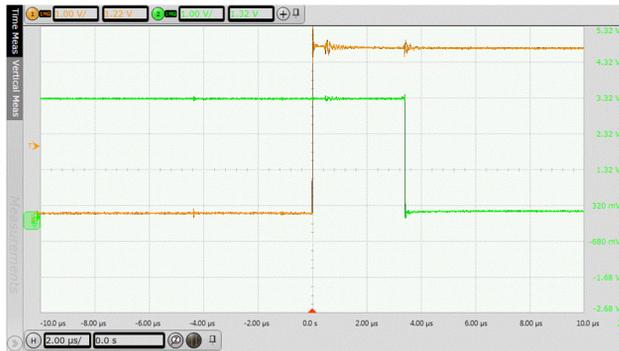
Figure 5: Response time of MIS loopback (Orange: Interlock Input, Green: Interlock Output).
