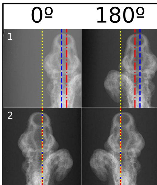
Figure 10: Iterations for sample alignment at 0 and 180 degrees. In yellow is the center of detector, blue is the axis of rotation and red is the center of the sample.
