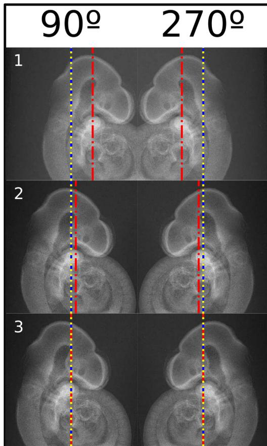
Figure 11: Iterations for sample alignment at 90 and 270 degrees. In yellow is the center of detector, blue is the axis of rotation and red is the center of the sample.
