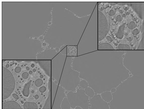
Figure 9: Artifacts from COR misalignment. Upper Square: Reconstruction with COR misaligned in 2 pixels. Bottom square: Reconstruction after alignment using the proposed process.
