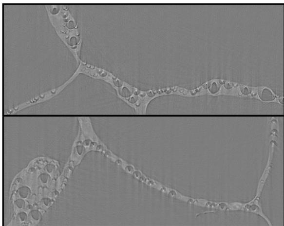
Figure 7: Artifacts from misaligned angles. Top image: Upper part of the sample (200 of 2048 slices). Bottom image: Bottom part of the sample (1848 of 2048 slices).
