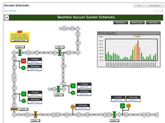
Figure 6: Vacuum display mock-up in Balsamiq.
