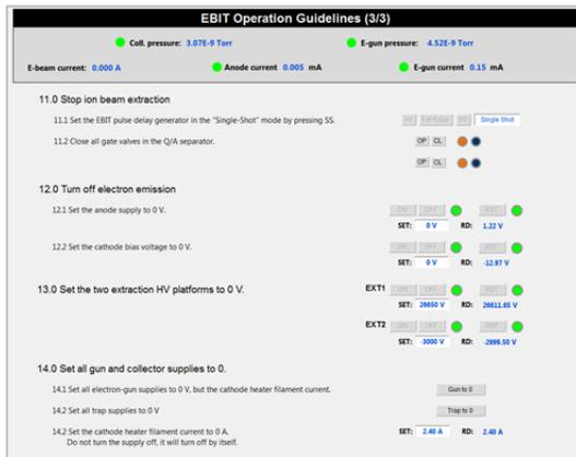
Figure 3: Specialized display with a guided walkthrough for starting the EBIT.
