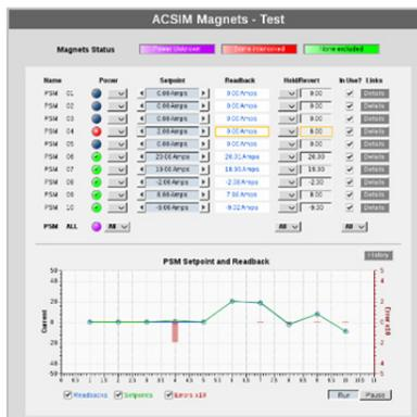
Figure 7: CS-Studio screen for simulated magnets.
