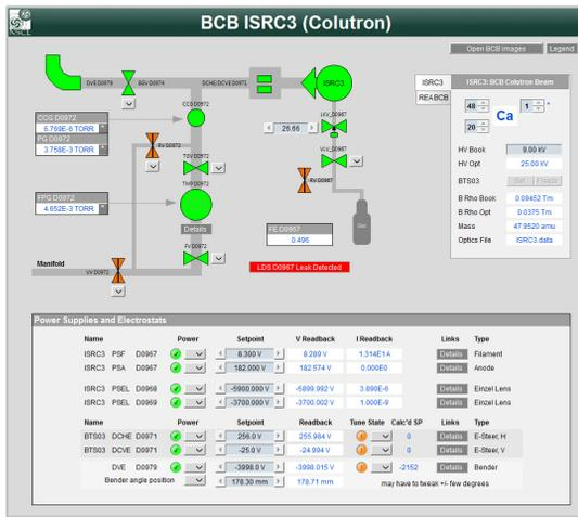
Figure 2: Specialized display for an ion source combining status and controls for vacuum, power supplies, gas leak and beam selection.
