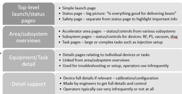
Figure 4: Hierarchical plan for interfaces: top level launch status, area/subsystem overviews, equipment/task detail, and detail support.
