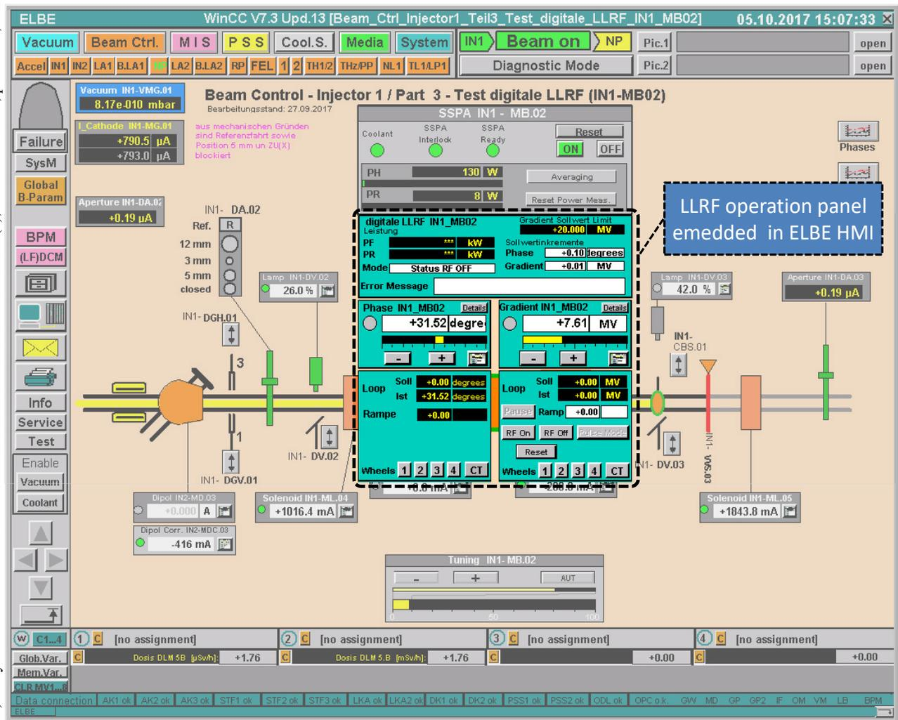
Figure 6: LLRF operation panel embedded in ELBE WinCC HMI.
