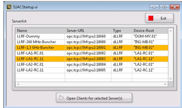
Figure 4: LLRF GUI start-up panel.
