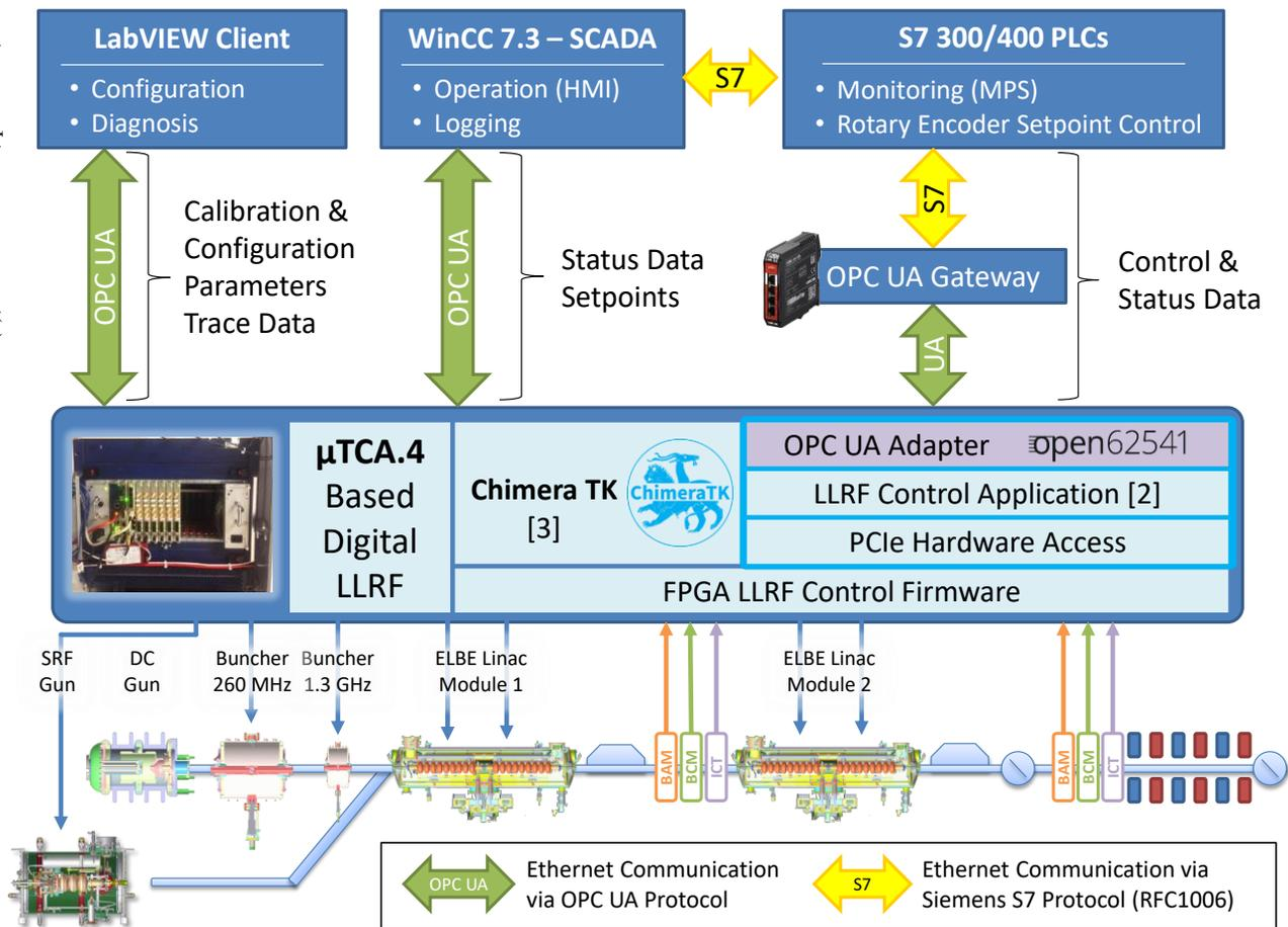
Figure 1: Digital LLRF ELBE control system integration scheme.
