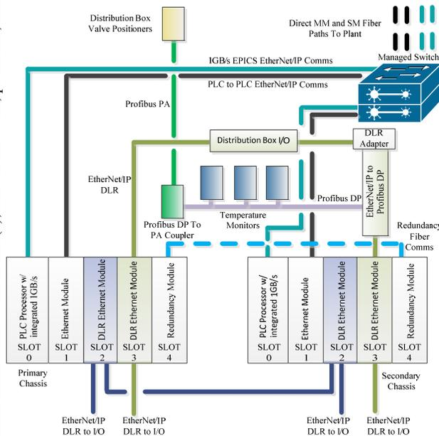
Figure 1: Centralized, redundant, PLC chassis.
