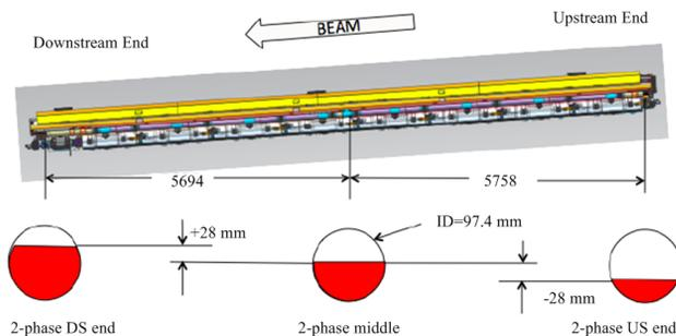
Figure 3: Liquid level for single LCLS-II cryomodule [6].
