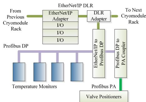
Figure 2: Typical networked controls hardware per cryomodule rack.
