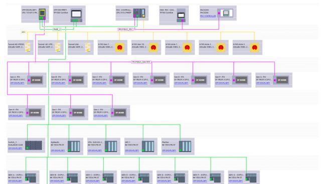
Figure 3: fragment of the AD control architecture showing the Profibus link (purple) between the PLC master and all PXIs slave, the Profinet link (green) for PLC slaves and the AS-i link (yellow) for safety slaves.
