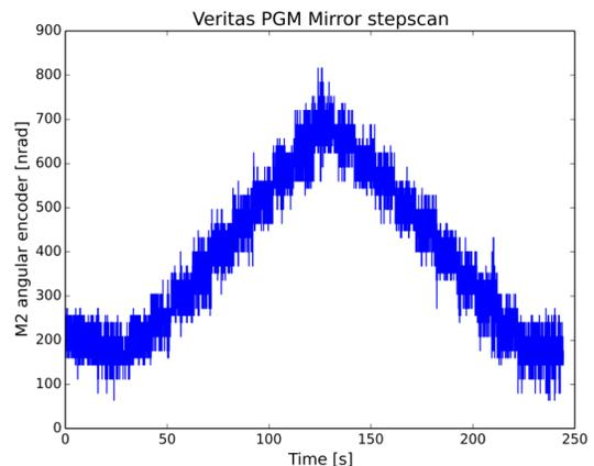
Figure 2: Veriat's monochromator mirror during a step scan of 10 up and down steps, with 10 seconds of sampling time in open loop.
