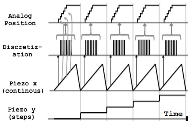
Figure 6: Time-based scan structure at Nanomax.
