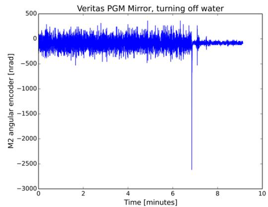
Figure 1: Noise in the monochromator mirror is reduced by a factor of five when the two valves controlling the flow are closed.
