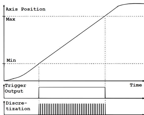
Figure 5: Min/max time based scan.
