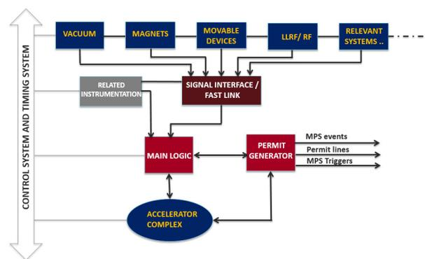
Figure 2: MPS integrated overview diagram.
