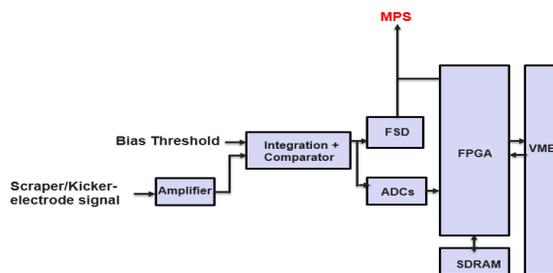
Figure 6: Electrode loss protection.
