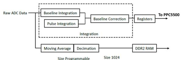
Figure 5: Ring pickup signal processing.
