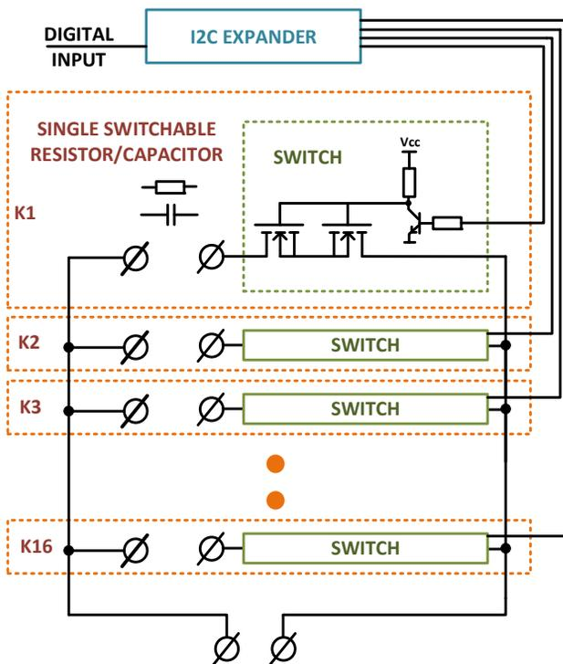
Figure 4: Single variable resistance / capacitance tuner block diagram.
