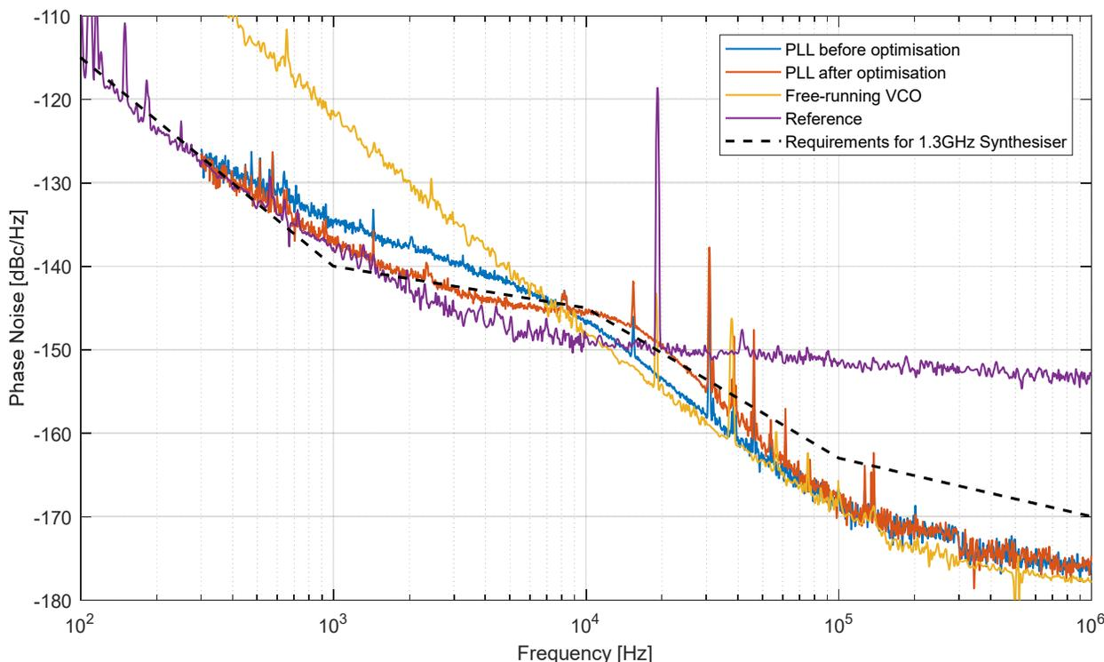
Figure 6: Compared phase noise measurements: reference signal, free-running VCO and PLL output signal for the optimised vector start and end values.
