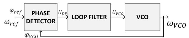
Figure 2: PLL block diagram.
