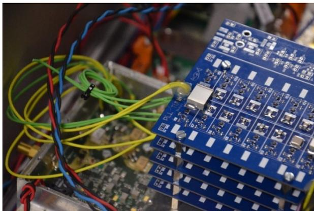
Figure 5: Tuners connected to the Master Oscillator 1.3 GHz Synthesiser PLL.
