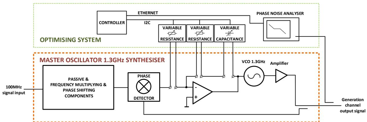
Figure 3: Block diagram of the optimising system.
