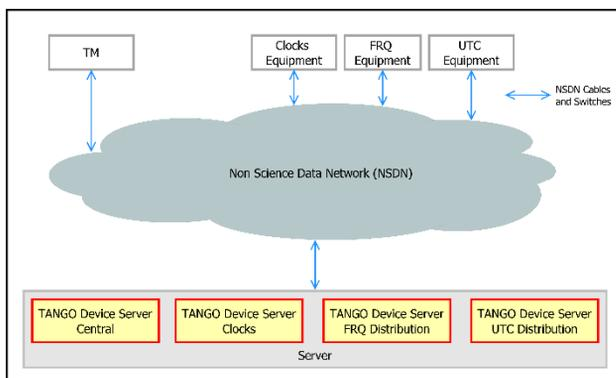
Figure 6: SAT.LMC-NSDN-SAT Logical Connectivity.
