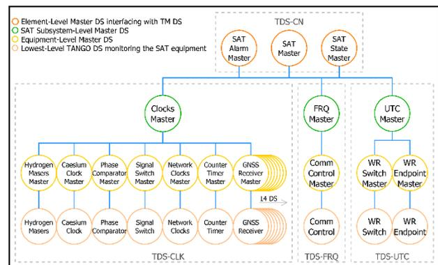
Figure 3: SAT.LMC TANGO Device Server Hierarchy.
