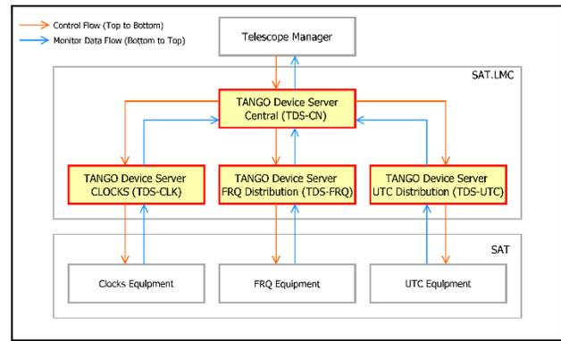
Figure 2: SAT.LMC Hierarchical solution.
