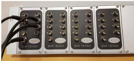
Figure 3: The multiplexers are mounted in 19" frames and can easily be collocated with other patch panels from MAX IV.
