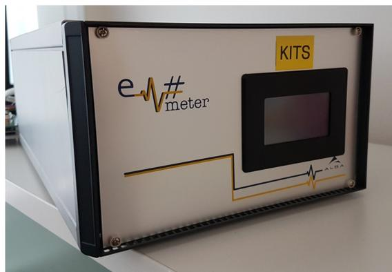
Figure 1: A touch panel is located at the electrometer front panel.
