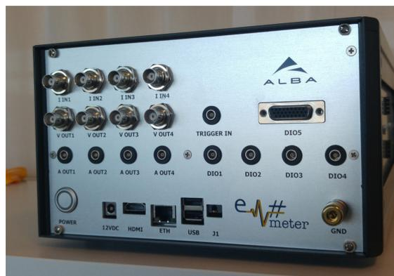
Figure 2: The back panel of the electrometer contains the interconnections such as input current, output voltages, trigger signals, I/O signals, together with the internal NUC computer ports.
