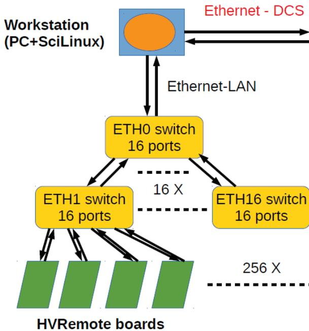
Figure 1: Architecture of the *HVRemote* control tree.
