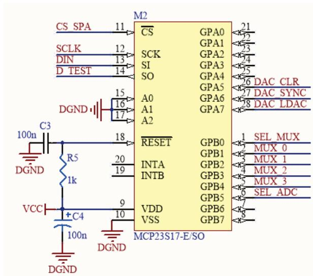
Figure 4: MCP23S17 signals in the *HVRemote-Ctrl* card.
