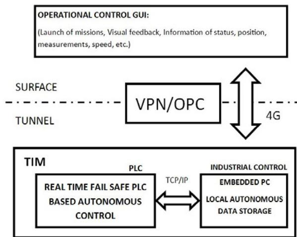
Figure 4: Overview of the control system with communication in between surface and tunnel.
