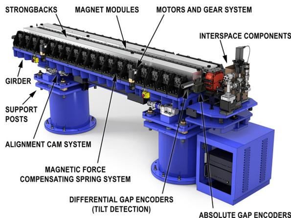
Figure 6: An LCLS-II Hard X-ray Undulator segment.
