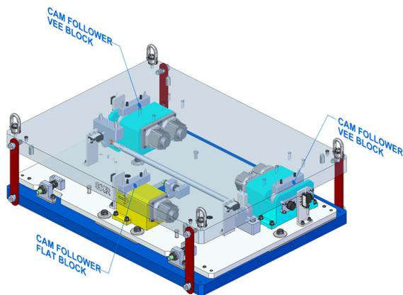
Figure 4: SXR interspace cam alignment system.
