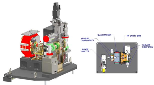
Figure 8: HXR interspace components, including RF cavity BPM, quadrupole magnet, vacuum components, and HXR phase shifter.
