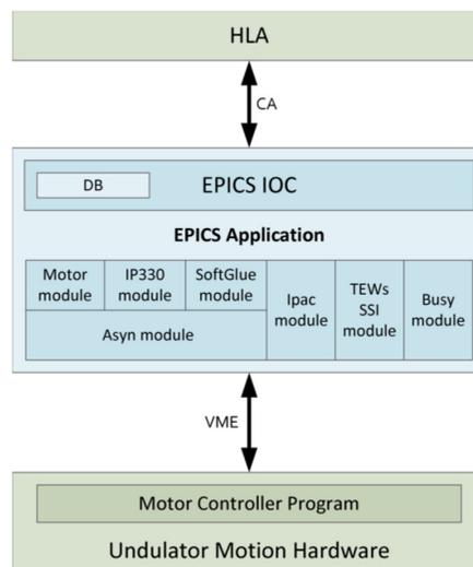
Figure 7: HXR software architecture overview, from high-level applications (HLAs) at the top to the undulator hardware at the bottom.
