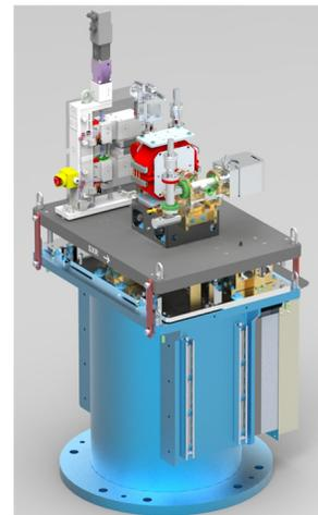
Figure 3: SXR interspace components on a pedestal, including from left to right: SXR phase shifter, quadrupole magnets, and RF cavity BPMs. The interspace motion controller can be seen mounted on the right of the pedestal.
