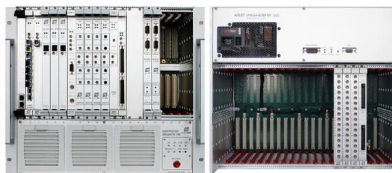
Figure 1: VME-BINP crate front and rear view.
