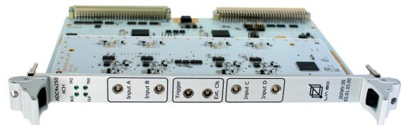
Figure 4: ADC4x250 4 channel version.
