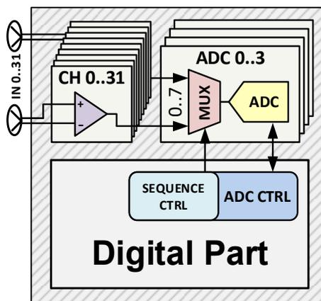
Figure 7: ADCx32 block diagram.
