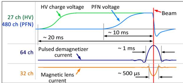
Figure 5: PHVS timing diagram.
