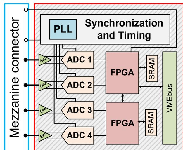
Figure 1: The structure of ADC4x250 mainboard.
