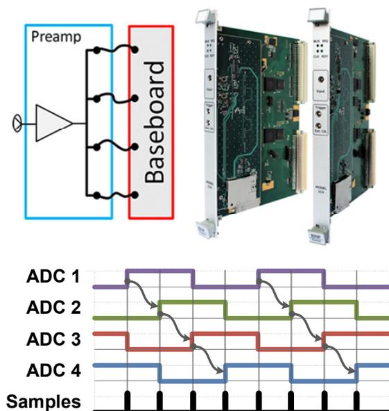
Figure 3: ADC4x250-1CH and its clock sequence.
