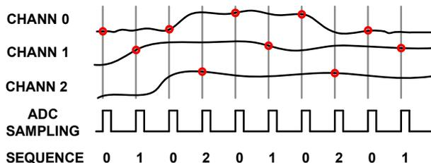
Figure 6: ADC channel sequencing.
