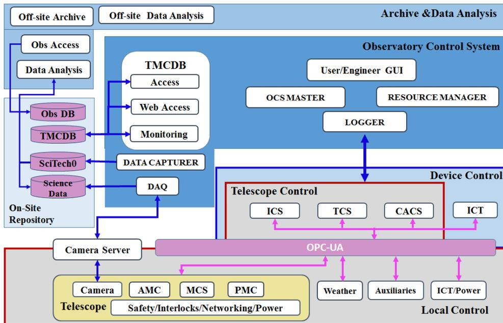
Figure 1: ASTRI SST-2M Control Software (MASS) architecture.
