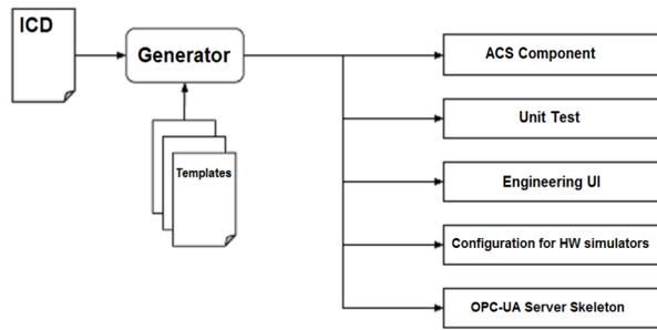
Figure 3: MASS code generation workflow.
