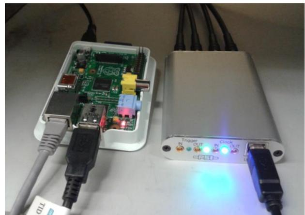
Figure 1: LHC clock monitor, able to detect misalignments of 100 ps.
