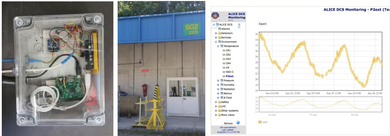
Figure 2: Weather station setup (left), installation point on the ALICE gas building (center), and a screenshot of the ALICE DCS monitoring web site (<http://alicedcs.web.cern.ch/AliceDCS/monitoring/main.aspx>), where temperature trends are published (right).
