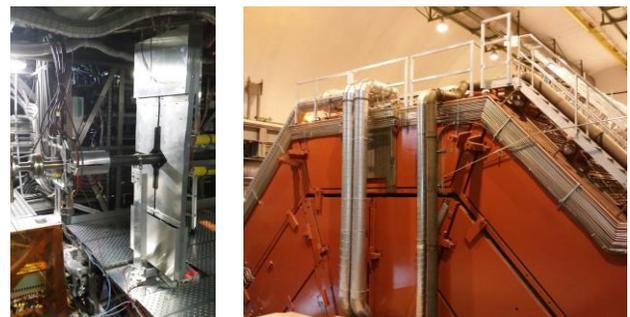
Figure 3: two installations of Raspberry Pi setups; left) near the interaction point, 1 m below the beampipe; right) on top of the ALICE L3 solenoid magnet.
