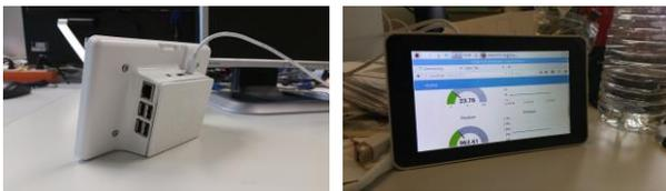
Figure 7: the last high-school students' project realized during summer 2017: a standalone setup composed by a Raspberry Pi 3 running Node-Red, a SenseHat shield with temperature and pressure sensors, a 7" touchscreen and a box enclosure.
