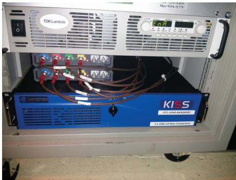
Figure 6: FEC and oscilloscopes used for arc detection in LHC.
