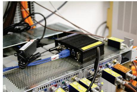
Figure 5: Equipment used to capture crowbar events.
