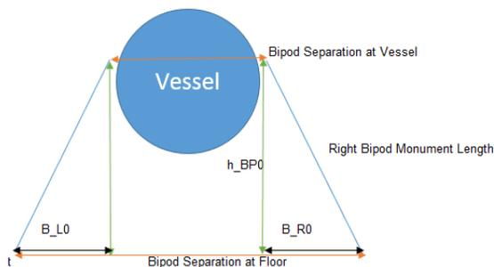
Figure 5: One component of the DIM kinematic model.
