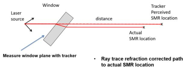
Figure 7: ATLAS Refraction Effect.
