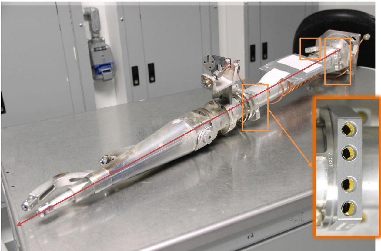
Figure 3: Diagnostic Snout with 12 ATLAS reflectors (orange boxes) and superimposed line of sight (red arrow). This diagnostic snout is approximately 1.2m in length. Four of the gold-coated retroreflectors are visible in the inset.
