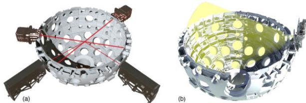
Figure 5: (a) the existing opposed port alignment system, (b) the wide field of view of the new ATLAS.
