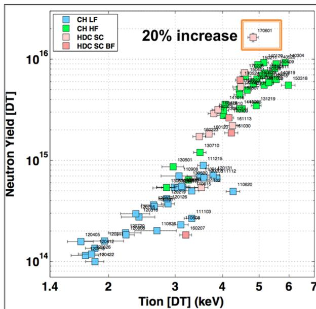
Figure 2: NIF ICF target experiment yield vs energy by platform.
