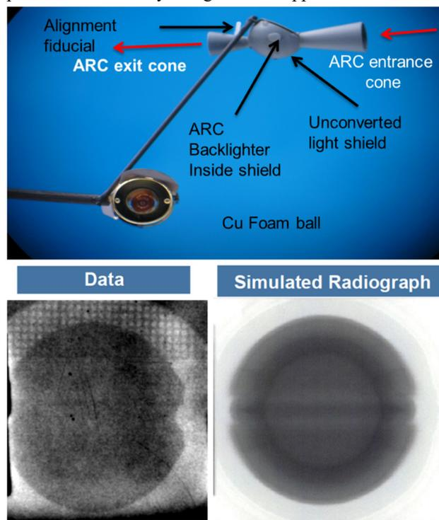
Figure 6: An example experimental target and ARC back-lighting target, with actual and simulated radiograph imagery obtained from recent experimentation.
