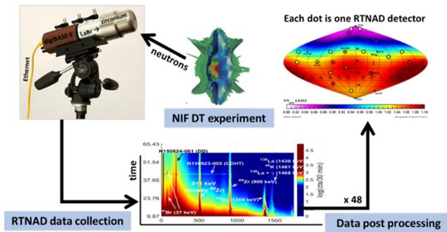
Figure 7: Control and data processing overview for the RTNAD diagnostic detectors.
