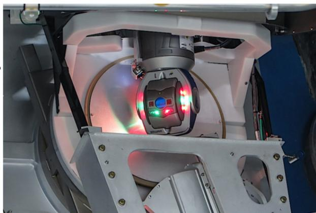
Figure 4: The ATLAS mounted on the NIF target chamber port performing self-calibration operation.
