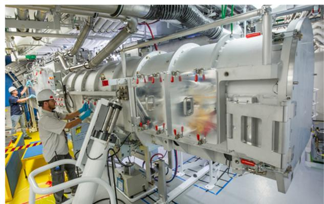
Figure 3: First of two new dual (target or diagnostic) positioners being prepared for a NIF shot.
