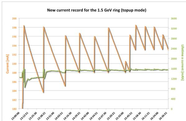
Figure 2: The figure shows top-up operation for a number of hours at the present maximum current. Plotted alongside the current is the product of current and lifetime.
