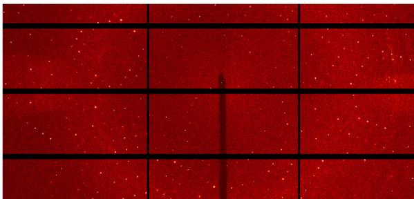
Figure 3: Diffraction patterns from crystals of the protein thaumatin exposed to X-rays produced by the new MAX IV 3 GeV storage ring. Collected with a Eiger XX M.
