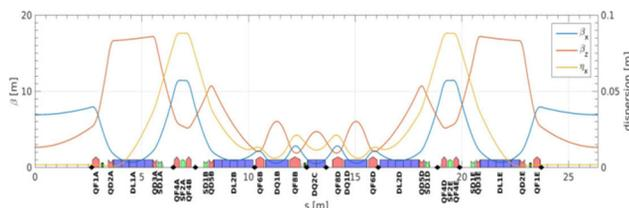
Figure 2: Arc cell optics layout.
