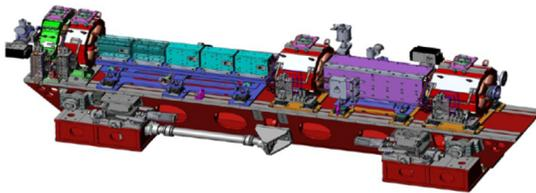
Figure 4: A motorized girder.
