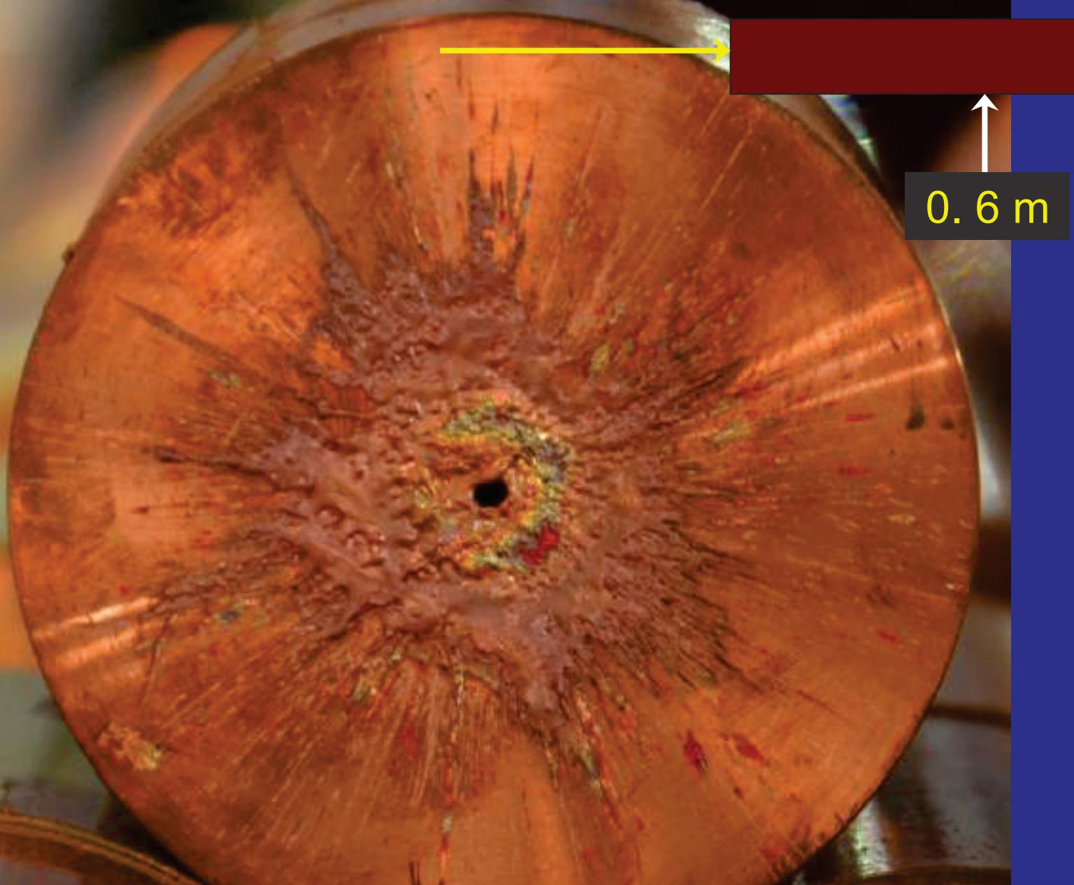
Hydrodynamic tunnelling: expected depth for FCC  $\sim 300$  m
