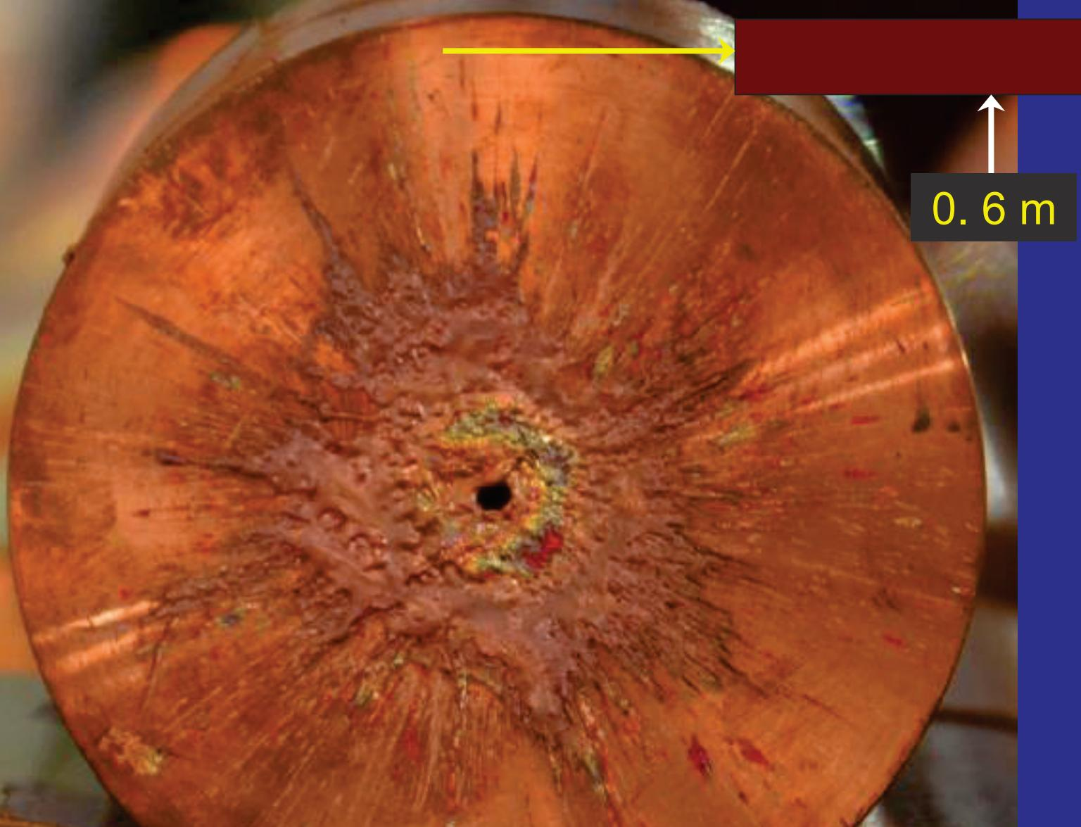
Hydrodynamic tunnelling: expected depth for LHC  $\sim 30$  m
