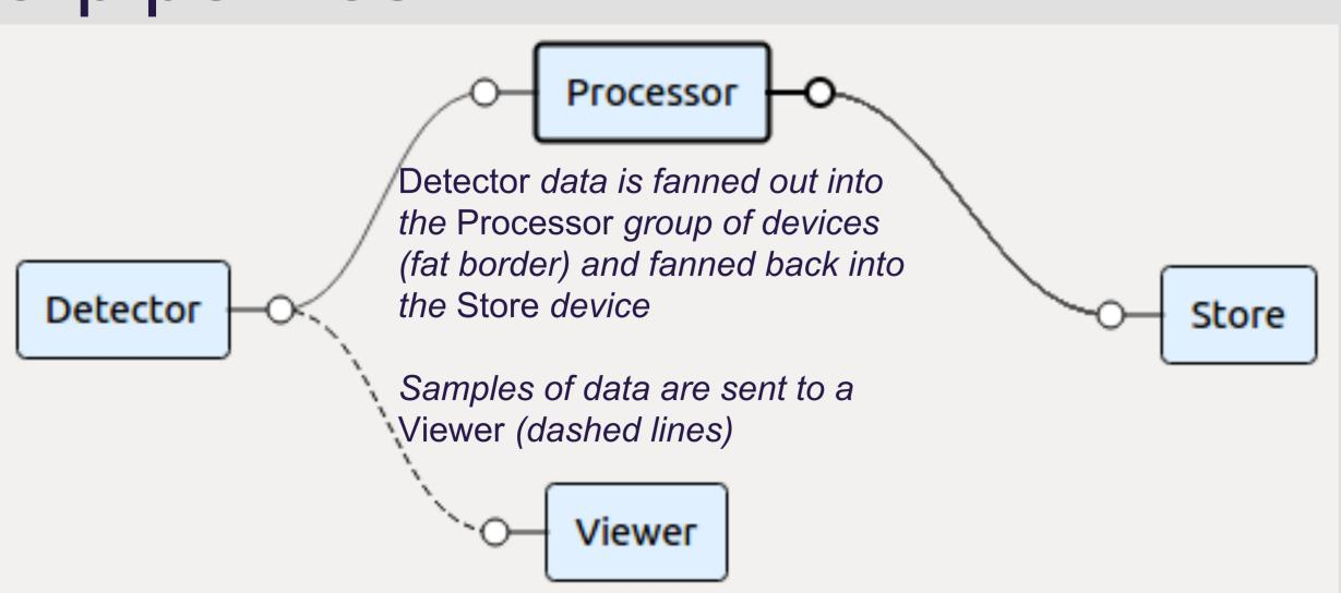
Karabo devices can communicate high-bandwidth data via direct links. These pipelines can be designed in the GUI as well.
