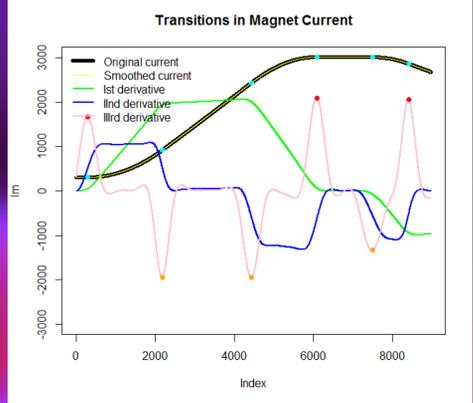
Above: Example of using R to develop an improved model to fit inductance data used in quench detector systems in RHIC.
