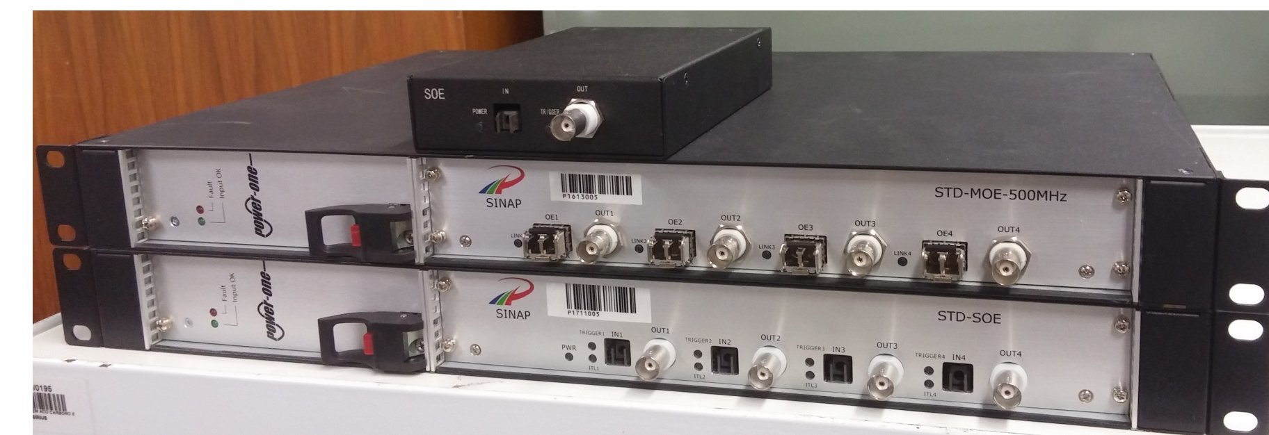
Figure 3: Optical to electrical converters developed by SINAP. Up to down are SOE, STD-MOE and STD-SOE.
