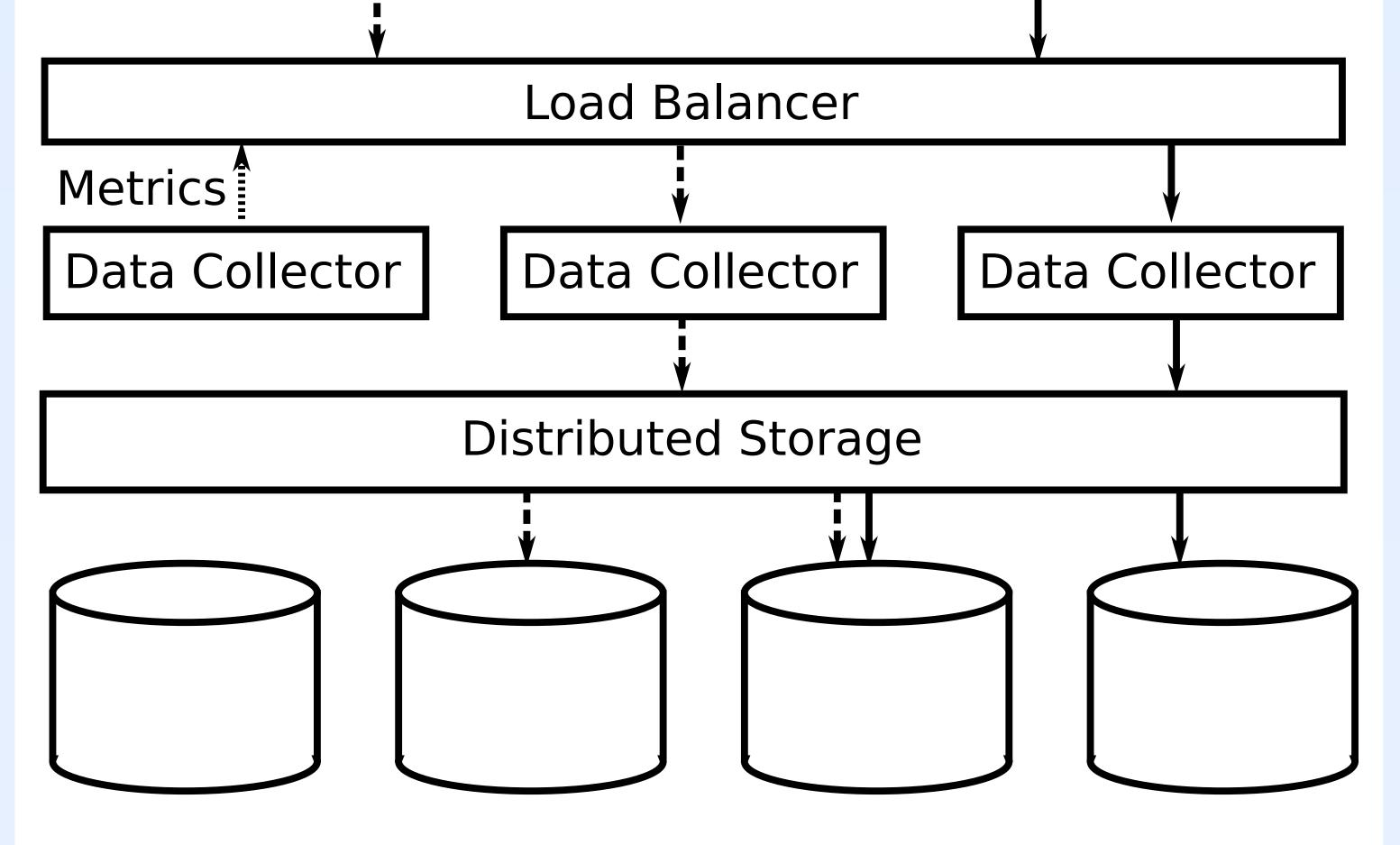
The targeted simplified Post Mortem architecture. Devices dump Post Mortem data to Data Collectors that are part of a load-balancing scheme. This way the load can be distributed among the Data Collectors of the Post Mortem cluster. The Data Collector that processes the dump writes the data to the distributed storage. The data are automatically replicated by the storage infrastructure.
