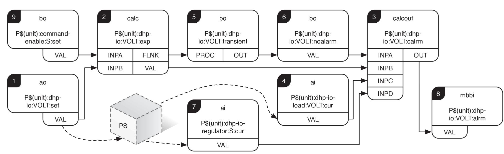
EPICS database structure to calculate alarms for a power supply channel.
