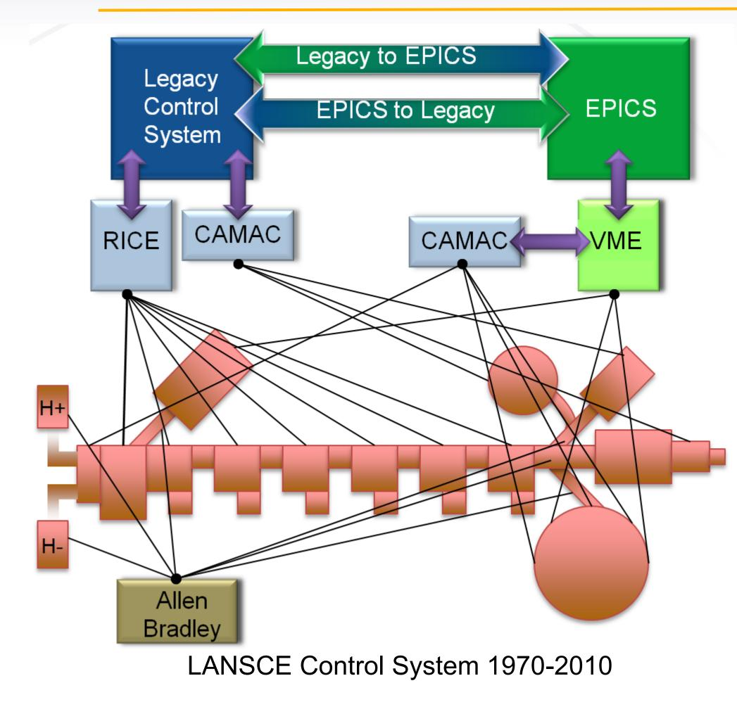
The LANSCE accelerator looks back at almost 45 years of operations. It was one of the first using computer technologies to control and monitor its beam line components. It started out with a custom in-house design called RICE (Remote Instrumentation and Control Equipment) which was installed in the early 1970's when the facility was built. Since then the facility has seen partial upgrades and extensions utilizing CAMAC, VME, and PLCs while introducing EPICS (Experimental Physics
