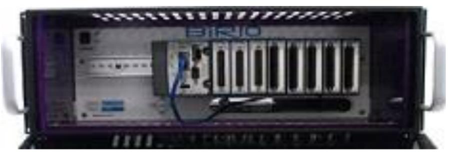
National Instrument CompactRIO (cRIO): reconfigurable control and acquisition system supported by EPICS. Real-Time Controller with 8-slots chassis and a user programmable Xilinx Virtex-5 LX110 FPGA) in the backplane interfacing to signal conditioning modules.
