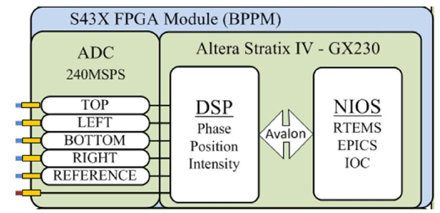
FPGA interfaced Mezzanine Card
