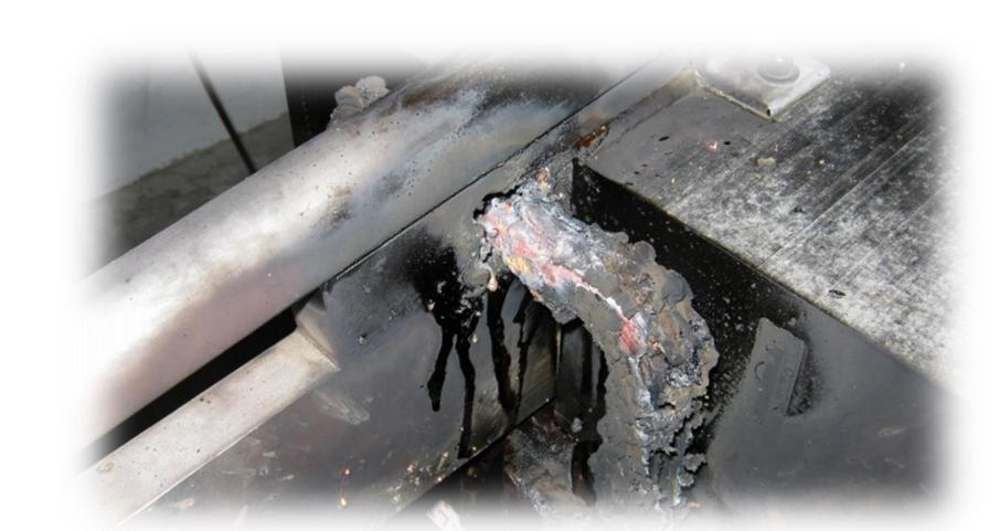
Preliminary modifications to the accelerator in 2011 for the forthcoming 12 GeV upgrade resulted in a YR septa magnet catching fire due to a lack of communication about machine readiness and was one of the motivating factors for creating a rigorous energized machine "pre-flight" readiness verification (hot checkout) process and supporting web application.
