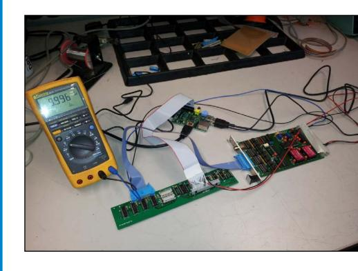
All booster magnet power supplies are driven by 16-bit DAC boards.
