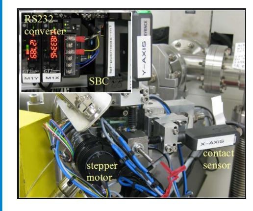
The software encoding of the stepper motors is imprecise due to slippage and x/y motion coupling. Therefore determination of the true mirror position must be realized by high-accuracy contact sensors and additional limit switches [26, 27].
