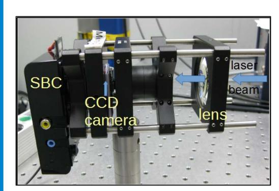
For near-field angle measuring of the beam guidance in the laser laboratory, a SBC, equipped with a standard 5-megapixel CCD camera, is in preparation. A converging lens focuses the beam on the CCD chip. Changes of beam angle yield a shift of the focal point of the Gaussian intensity distribution [33].
