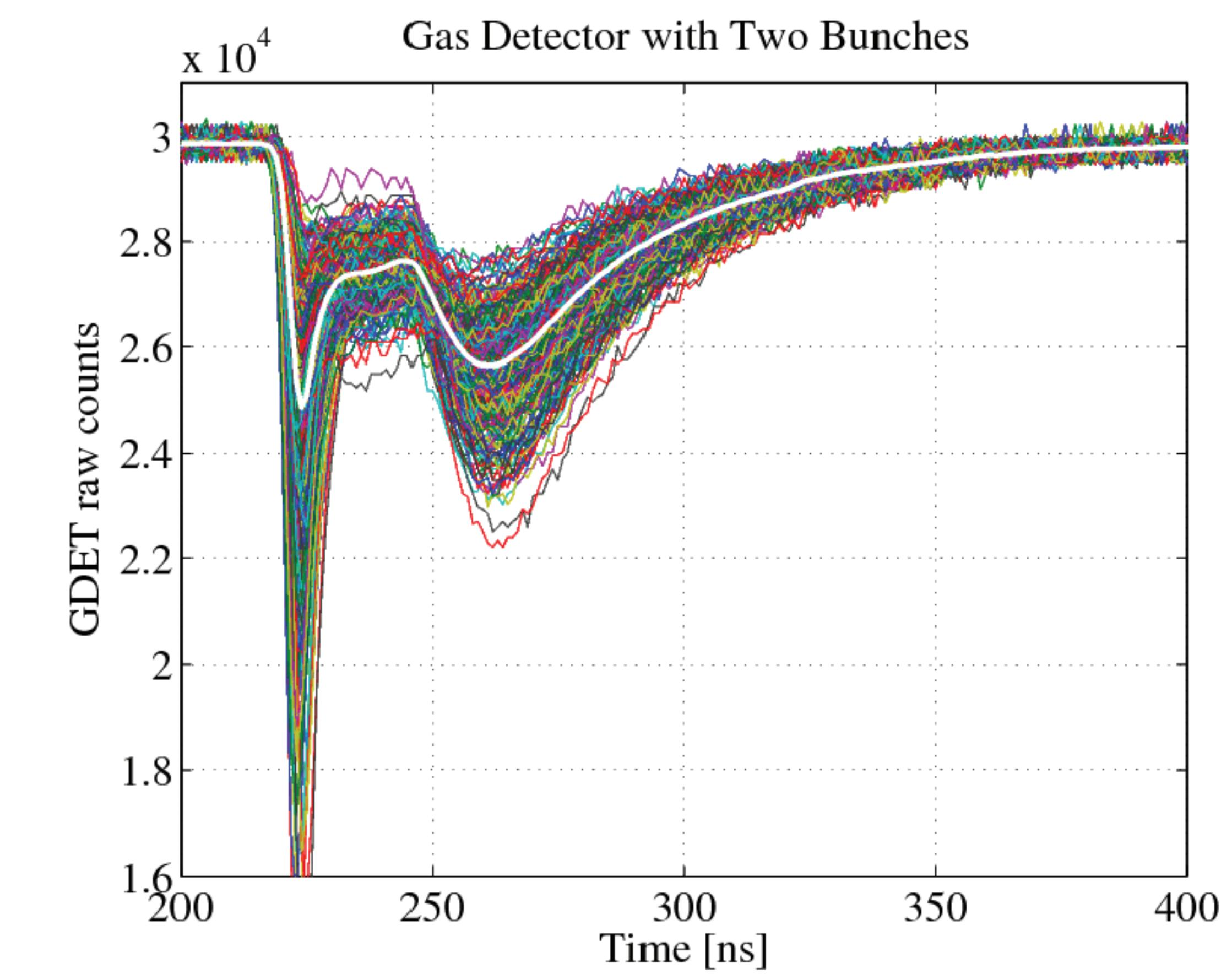
Gas Detector raw waveforms (above) show a 2.5:5 ratio after the laser heater was timed for the first bunch. The spike in the front is an instrumental reaction to coherent synchrotron radiation. Therefore the integrated GDET signal typically uses the counts from 250 to 400 ns.
