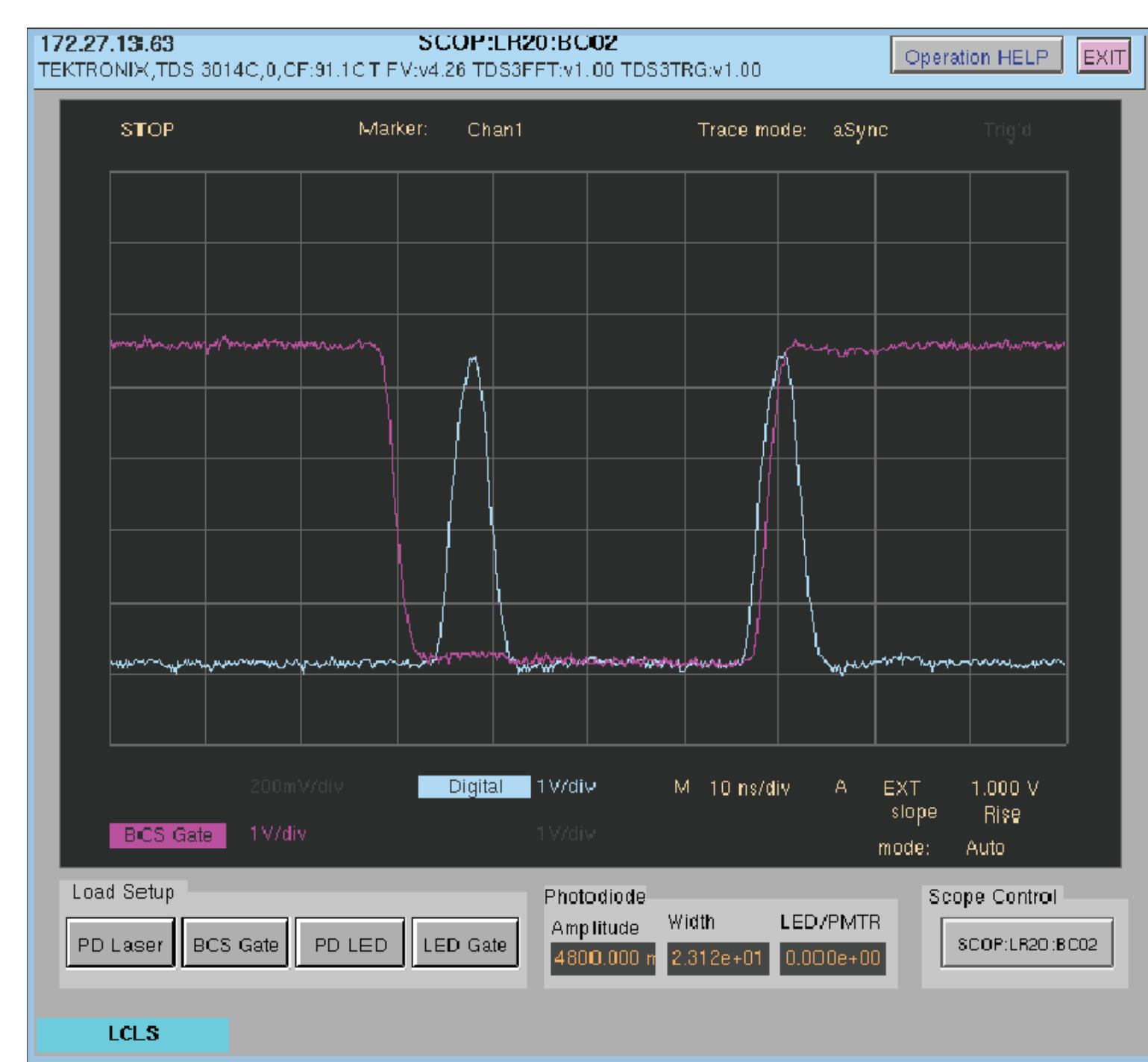
An optics box containing redundant beam splitters and photodiodes was used within the BCS Safety System to ensure that both laser pulses fell within the timing gate used by the Toroid Comparators downstream. Magenta trace shows the toroid timing gate and the blue trace shows the two laser pulses.
