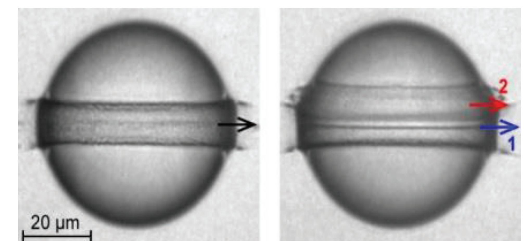
XFEL beams imaged by camera in CXI experimental hutch hitting water droplets. Single bunch beam is seen on the left and two-bunch on the right. The arrows indicate the XFEL beams.
