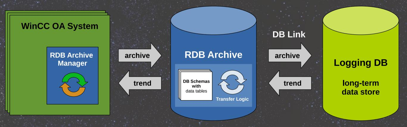
• Single high-performance RDB Archive Manager writes data to central Oracle DB • Data requiring long-term storage is transferred over a DBLink to the LoggingDB • Standard database transfer job mechanism, used by other LoggingDB clients, serves all applications and provides diagnostic and statistical information • Data stored in the LoggingDB can be made available in WinCC OA transparently
