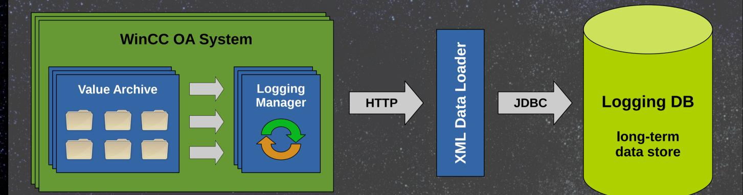
• Several WinCC OA Value Archive managers write historical data to local disk files • Custom WinCCOA LoggingManager programs query data, transform to XML and send to a dedicated data loader application of the LoggingDB service • The architecture would not scale to meet the new requirements for LHC Run II
