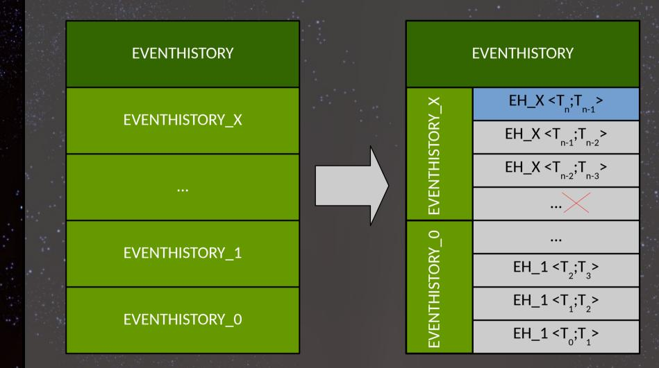
• Growing IOT leads to degraded query performance • Time-based partitioning (partition pruning) • Queries on views with pushed-predicate hints • Data retention policy (3 months in daily partitions) Automated partition-managent job for 200 schemas
